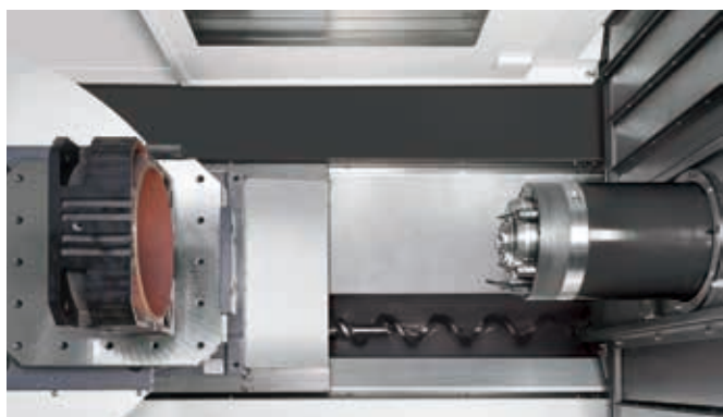
One piece Z-axis cover + Screw chip remover
