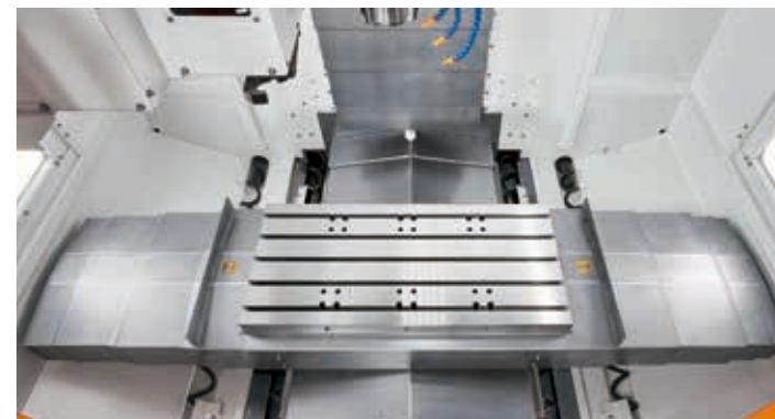
Bottom guarding flush + Screw chip removers
