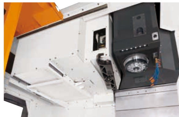
Arm type ATC + Auto door for magazine + Coolant ring + LED lights
