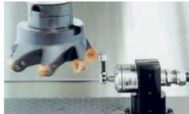
Auto tool length measurement
