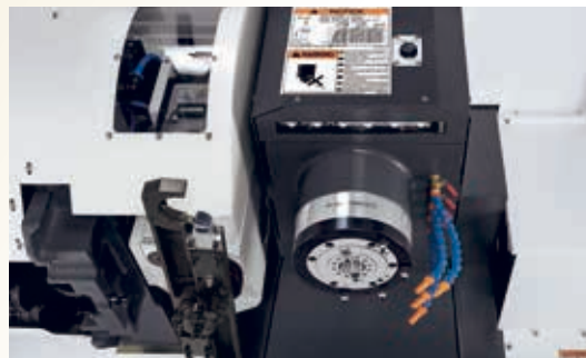
Arm type ATC + Coolant ring + LED lights
