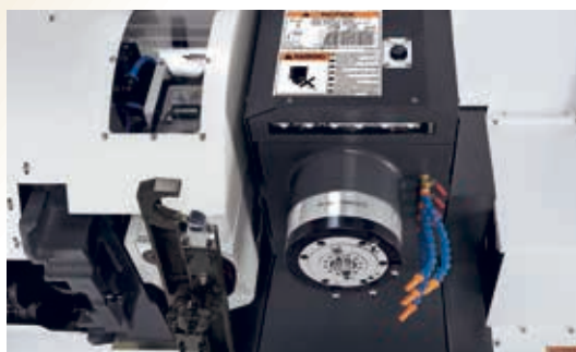
Arm type ATC + Coolant ring + LED lights
